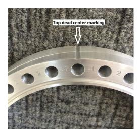
The second wedge should be installed with the numbered side facing towards the nozzle side with top dead center mark in its highest possible position. This is 0 DEGREES.
